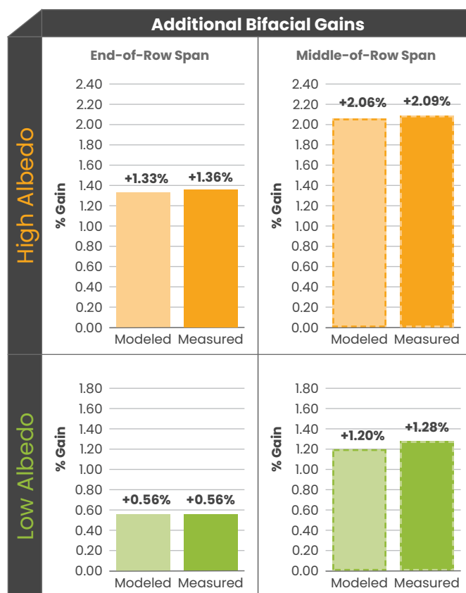
FIGURE 9 The close fit between the modeled versus measured NX Horizon bifacial gain advantage as compared to the other 1P single-axis tracker design validates the iteratively determined loss factors, detailed in Figure 8, for the end- and middle-of-row spans.
