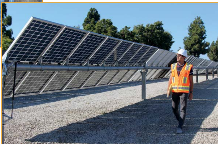
HIGH-ALBEDO CONDITION By installing a white fabric, researchers are able to characterize bifacial performance under high-albedo conditions. This white fabric—which is alternately installed or removed on a monthly basis—has an albedo of roughly 50%.
