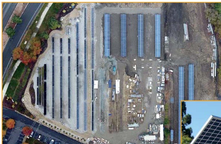
CENTER FOR SOLAR EXCELLENCE Nextacker’s bifacial testbed in Fremont, California, consists of five 1P tracker rows and four 2P tracker rows. Test hardware includes bifacial modules from three different vendors.
