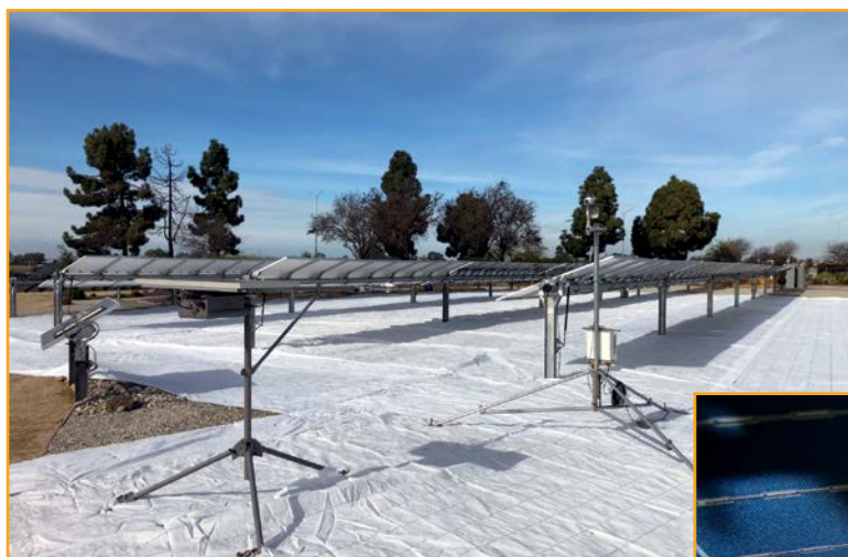
HIGH-ALBEDO CONDITION By installing a white fabric, researchers are able to characterize bifacial performance under high-albedo conditions. This white fabric—which is alternately installed or removed on a monthly basis—has an albedo of roughly 50%.
